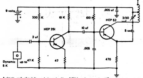
A simple, early circuit for a wireless mic. Use a 3/8" form for the coil and IB enameled wire; wind seven turns, tap at number two. Frequency can be vaired by adding or subtracting from coil. The first transistor is an audio amp (any good audio type will suffice) and the second an rf oscillator (again, any like type will work).
