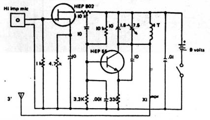
Wireless mic for commerical FM band. Tuning is accomplished by adjusting the variable cap. XI is made by twisting 2 inch lengths of small guage insulated wire together. Should give range of 2 blocks to 3 mile with good receiver. In any wireless mic a condenser mic can be substituted for the dynamic variaty by simply adding a line to the power source as shown in the directions for the mic, this will give increased pick-up.
