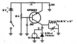
Ultra sub-mini transmitter uses modern circuit with a Poly Paks varactor to achieve FM modulation. Transmits about 300 ' In the commerical FM band directly from tank circuit. 3' antenna can be added to tank coil and for greater range. For super amall power supply disassemble a 9 volt battery and use on bank of cells.
