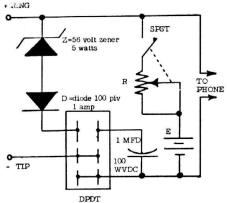
E=6-24 volt battery R=1 KOhm Pot, audio taper with on-off switch The standard 10 K ohm resistor is <u>NOT</u> needed. The capacitor passes the audio but blocks the DC voltage which results in an "on-hook" condition. The 1 K ohm pot gives you a level control for <u>YOUR</u> voice. And speaking of Black Box modifications here's a circuit control from Brooklyn N X on how to connect
