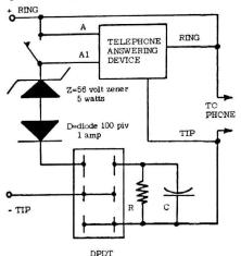
R=10 KOhm resistor, 1/2 watt C=1 MFD capacitor, 100 wvDC
