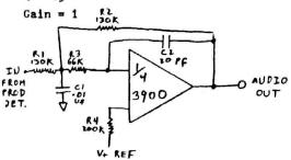
R1 and R2 should be 100K for a 15KHZ cutoff R3 should be 53K for a 15KHZ cutoff
