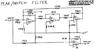
IF FILTER IS NOT NOTES ALL CAPACITORS FOR FILTERS 15.738 KHZ, ADJUST THE SILVER MICA 2 - 100K RESISTORS.
