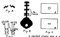
A warded plate has a slit in it (see fig. C-A), while a open plate has a hole in it (see fig C-B). Thus be mixing the plates a key combination is made up. For every warded plate there is a cut in the key. By the way fig. A is a cross section of the two different types of keys. The only difference between them is the direction of the
