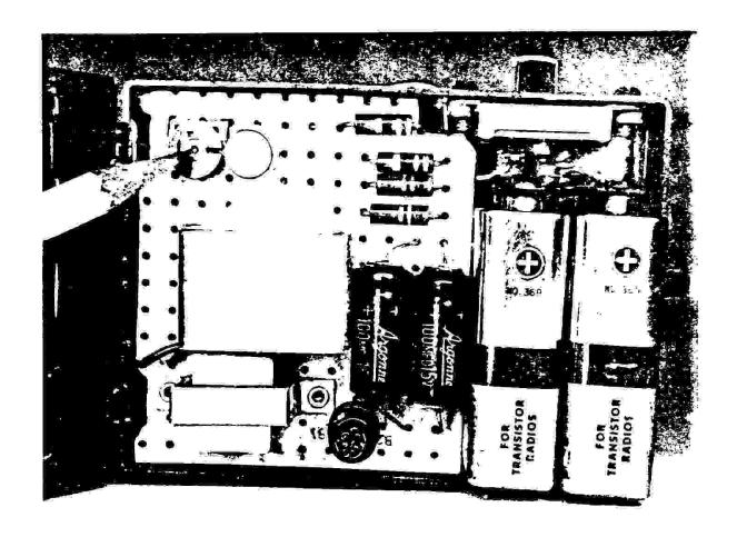
The parts layout is not critical, the author's unit was assembled in a plastic box. A subminiature pot allows feedback adjustment for oscillation of transstor Q2.
