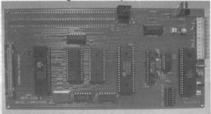
The replica I is a functional clone of the apple I computer. It includes a 65C62 MCU running at 1MHz, 32K RAM and 6K ROM with monitor built in. The replica has built in video and the capability to use an authentic ASCII keyboard or more modern PS/2 keyboard. Simply add a standard PC style AT power supply, keyboard and NTSC composite TV or monitor. Add the optional serial I/O interface and you can store and load programs from any PC. Kits start at just \$199.
