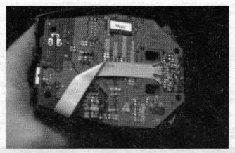
Figure 4. Connection soldered to the underside so the original palm connector is still available for use.
