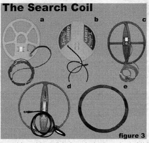
When you purchase a metal detector it has a coil already mated and ready to go into the field. But there are a few companies that focus on manufacturing after market search coils which can be a big improvement over some stock coils. The coil is mounted to the support shaft with a nylon type bolt and wing nut and can be tilted forward and backward to get the proper angle to sweep with. (See Figure 3)
