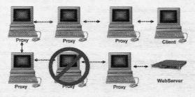
Example of working chain that will simply not work at all (Remember this. "A proxy chain is only as strong as the weakest link" \*2)
