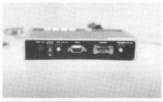
Backside of the scrambler showing the 9-pin D-Sub connectors, mic and speaker volume adjusts, power connector, and fuse holder.
