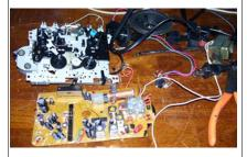
As you can see, I definitely got my money's worth out of it. I salvaged an AC power cord, 6V transformer, telescoping whip antenna, a cassette deck with motors, gears, and other mechanical bits, and a circuit board with some useful RF parts including an AM looopstick antenna, tuning capacitor, and some inductors.
