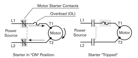
Melting AlloyOne method of providing overload protection is with a melting<br/>alloy overload relay. The alloy is a solder which melts at a very<br/>precise temperature. When it reaches this specific temperature<br/>it will change from its solid state to a liquid state. This<br/>temperature never changes, ensuring the accuracy of the<br/>overload during the life of the relay.
