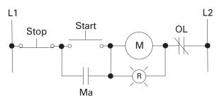
When the coil is energized, the light will illuminate to indicate the motor is running. In the event the pilot light burns out the motor will continue to run.
