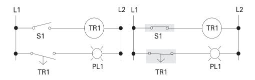
When S1 is opened, TR1 begins timing. When 5 seconds has elapsed, TR1 will open its associated normally open contacts, extinguishing pilot light PL1.
