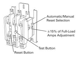
The Siemens Sirius 3RU11 is a bimetal type of overload relay with the heater elements as an integral part of the design. The unit comes with a Class 10 trip as standard. The Sirius 3RU11 features manual or automatic reset, adjustable current settings, and ambient compensation. A switch-position indicator also incorporates a test function which is used to simulate a tripped overload relay. A normally open and a normally closed auxiliary contact are included.
