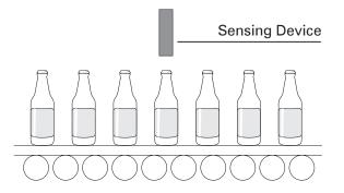
Short switching times allow it to perform high-speed counting for speed monitoring.
