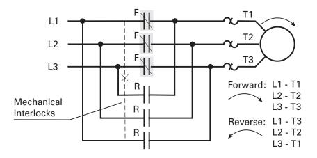
When the "R" contacts are closed, current flows through the motor in the opposite direction causing it to rotate in a counterclockwise direction. Mechanical interlocks prevent both forward and reverse circuits from being energized at the same time.
