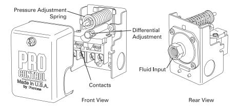
The basic components of a pressure switch are illustrated below. Electrical contacts are operated by the movement of a diaphragm against the force of a spring. The contacts may be normally open (NO) or normally closed (NC). The spring setting determines how much fluid pressure is required to operate the contacts.
