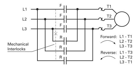
When the "F" contacts are closed, current flows through the motor causing it to turn in a clockwise direction.
