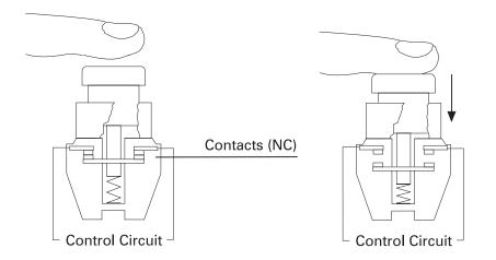
Pushbuttons are available with variations of the contact configuration. For example, a pushbutton may have one set of normally open and one set of normally closed contacts so that when the button is depressed, one set of contacts is open and the other set is closed. By connecting to the proper set of contacts, either a normally open or normally closed situation exists.
