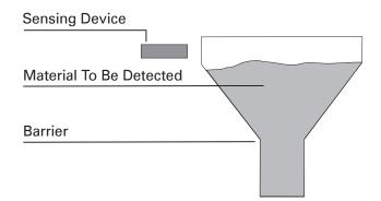
The following chart illustrates the proper capacitive proximity switch when detecting material through a barrier.
