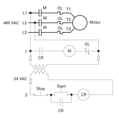
When the "Start" pushbutton in line 2 is momentarily depressed, power is supplied to the control relay (CR).
