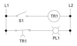
When S1 is closed, timing relayTR1 is energized. After a timed delay of 5 seconds, the associated normally closedTR1 contacts open, extinguishing PL1. When S1 is open, deenergizingTR1, theTR1 contacts close immediately, illuminating PL1.
