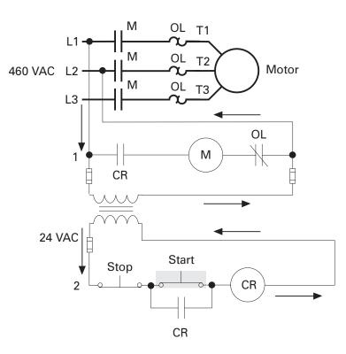
The "CR" contacts in lines 1 and 2 close. The "CR" contacts in line 2 maintain the start circuit. The "CR" contacts in line 1 complete the path of current to the "M" motor starter. The "M" motor starter energizes and closes the "M" contacts in the power circuit, starting the motor. Depressing the "Stop" pushbutton deenergizes the "CR" relay and "M" motor starter.
