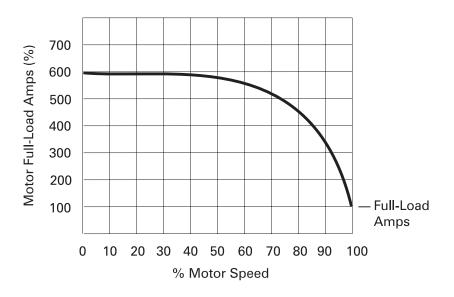
Another potential problem with applying full-voltage starts is the high torque developed when power is first applied to the motor. This can be as high as 175% to 200% of full-load torque on a standard NEMA B type motor. Many applications require the starting torque to be applied gradually. A conveyor belt, for example, requires the starting torque to be applied gradually to prevent belt slipping or bunching.
