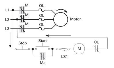
When the object to be detected comes in contact with the actuator, the limit switch will open. The "M" contactor is deenergized and the motor stops. The motor can be manually restarted when the object is no longer in contact with the actuator and the limit switch is closed.
