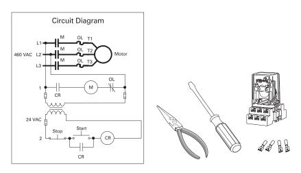
Many of the same tasks can be performed with LOGO!. Initial hard-wiring, though still required, is greatly simplified. Modifying the application is as easy as changing the program via the keypad located on the front of the LOGO!. Likewise, control programs can be created and tested before implementation via a PC software program. Once the program is performing per specification, the transfer to LOGO! is as simple as plugging in a cable.
