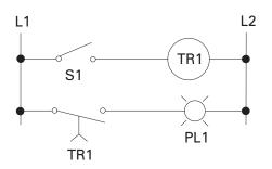
When S1 is closed, TR1 begins timing. When 5 seconds has elapsed, TR1 will close its associated normally open (NO) TR1 contacts, illuminating pilot light PL1. When S1 is open, deenergizing TR1, the TR1 contacts open immediately, extinguishing PL1.
