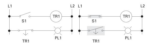
When S1 is opened, timing relay TR1 is deenergized. After 5 seconds, the associated normally closed contacts close, illuminating PL1.
