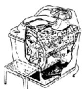
prevent odors. Electric models have a fan to assist venting and thermostat controlled heating element keep the floor of the chamber hand warm to assist evaporation. (Fans can be added to non-electric models.)
