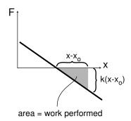
n / The area of the shaded triangle gives the work done by the spring as the cart moves from the equilibrium position to position x.
