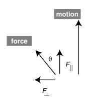
k / Work is only done by the component of the force parallel to the motion.
