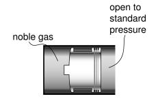
f / A simplified version of an ideal gas thermometer. The whole instrument is allowed to come into thermal equilibrium with the substance whose temperature is to be measured, and the mouth of the cylinder is left open to standard pressure. The volume of the noble gas gives an indication of temperature.
