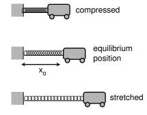
m / The spring does work on the cart. (Unlike the ball in section 3.1, the cart is attached to the spring.)
