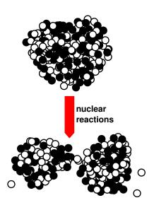
f / This figure looks similar to the previous ones, but the scale is a million times smaller. The little balls are the neutrons and protons that make up the tiny nucleus at the center of the uranium atom. When the nucleus splits (fissions), the potential energy change is partly electrical and partly a change in the potential energy derived from the force that holds atomic nuclei together (known as the strong nuclear force).
