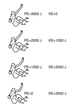
d / As the skater free-falls, his PE is converted into KE. (The numbers would be equally valid as a description of his motion on the way up.)
