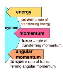
I / Energy, momentum, and angular momentum can be transferred. The rates of transfer are called power, force, and torque.
