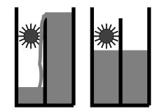
n / Entropy can be understood using the metaphor of a water wheel. Letting the water levels equalize is like letting the entropy maximize. Taking water from the high side and putting it into the low side increases the entropy. Water levels in this metaphor correspond to temperatures in the actual definition of entropy. Entropy is additive.
