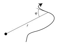
x / The  $r - \phi$  representation of a curve.
