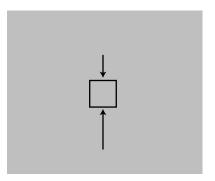
c / This does happen. The sum of the forces from the surrounding parts of the fluid is upward, canceling the downward force of gravity.
