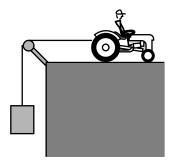
b / The tractor raises the weight over the pulley, increasing its gravitational potential energy.
