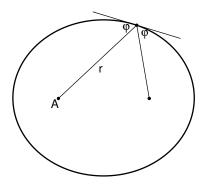
y / Proof that the two angles labeled  $\varphi$  are in fact equal: The definition of an ellipse is that the sum of the distances from the two foci stays constant. If we move a small distance  $\ell$  along the ellipse, then one distance shrinks by an amount  $\ell \cos \varphi_1$ , while the other grows by  $\ell \cos \varphi_2$ . These are equal, so  $\varphi_1 = \varphi_2$ .
