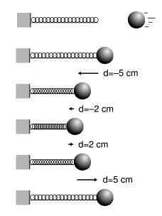
g / Whenever energy is transferred out of the spring, the same amount has to be transferred into the ball, and vice versa. As the spring compresses, the ball is doing positive work on the spring (giving up its KE and transferring energy into the spring as PE), and as it decompresses the ball is doing negative work (extracting energy).
