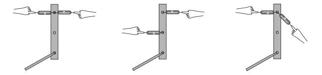
While one person holds the pencil which forms the axle for the ruler, the other members of the group pull on the scale and take readings. In each case, calculate the total torque on the ruler, and find out whether it equals zero to roughly within the accuracy of the experiment.
