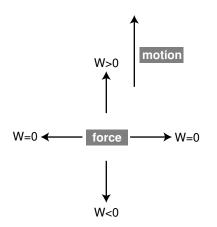
j / A force can do positive, negative, or zero work, depending on its direction relative to the direction of the motion.
