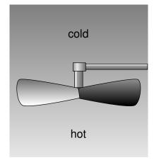
h / The temperature difference between the hot and cold parts of the air can be used to extract mechanical energy, for example with a fan blade that spins because of the rising hot air currents.
