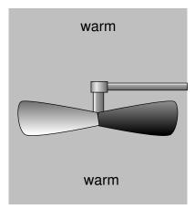
i / If the temperature of the air is first allowed to become uniform, then no mechanical energy can be extracted. The same amount of heat energy is present, but it is no longer accessible for doing mechanical work.
