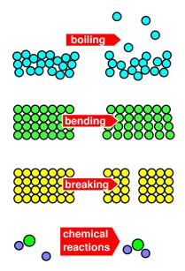
e / All these energy transformations turn out at the atomic level to be changes in potential energy resulting from changes in the distances between atoms.
