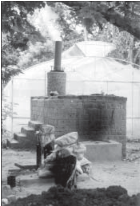
Steam curing plant (capacity:1300 blocks per shift)
