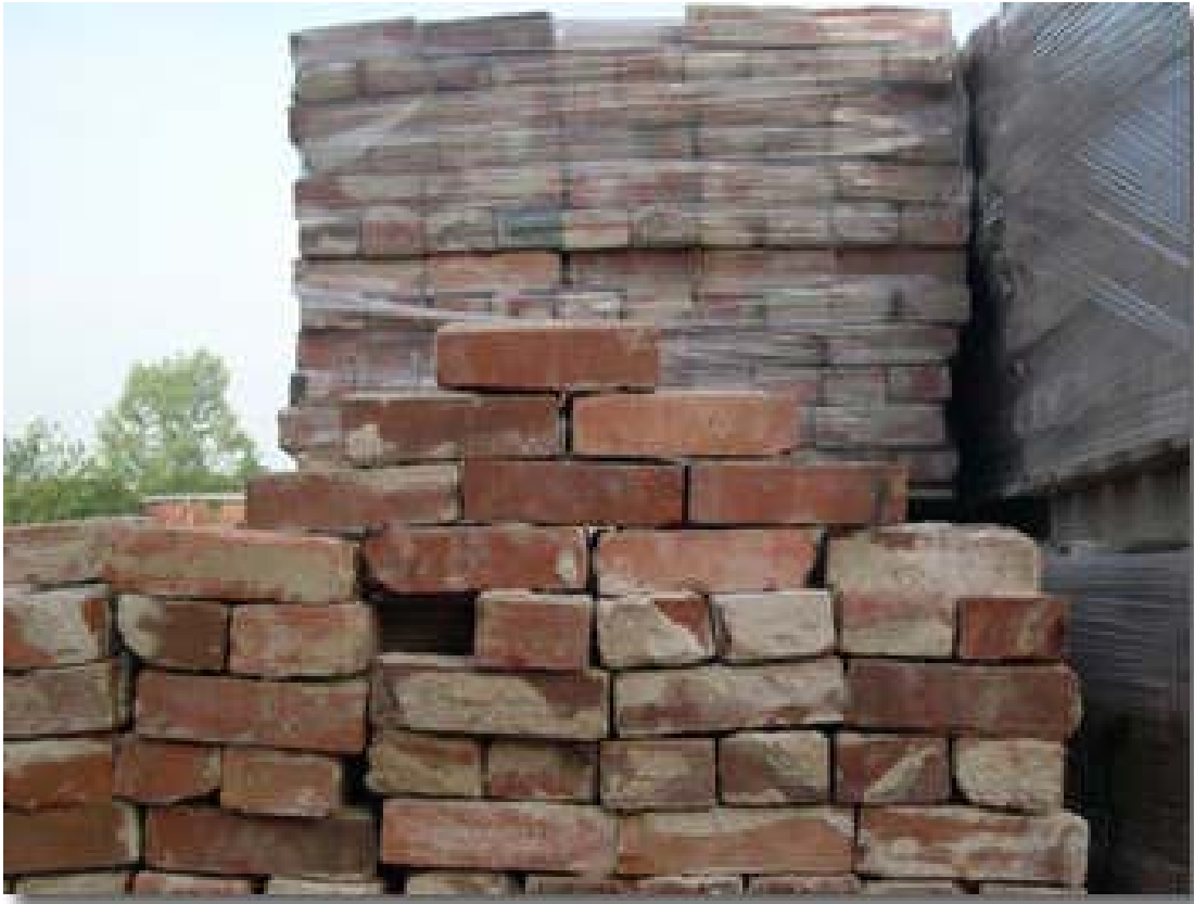
Figure 10. Pallets of salvaged bricks.
