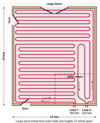
I felt that 2 inches would be too thin, and the concrete contractor refused to pour less than 3 inches due to the risk of damaging or exposing the tubing. The 3 inches still allows me to use a single household thermostat to control the heating, though it is less responsive. I'm still testing, but I believe that the system can raise the building temperature by about 3°F (1.6°C) per hour.
