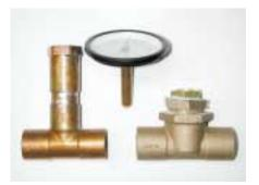
A brass seat tee with reducer (right) keeps the thermometer sensor in the fluid's flow. Copper fittings (left) don't work as well.
