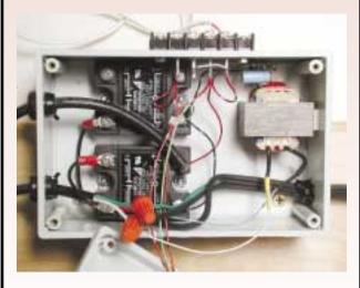
A homebuilt, solid-state relay box allows standard thermostats to control the system's AC circulation pumps.
