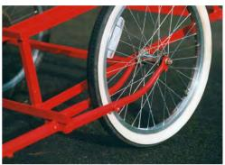
The next part is the towing bar. It needs to line up exactly with the left hand rear wheel mount.
