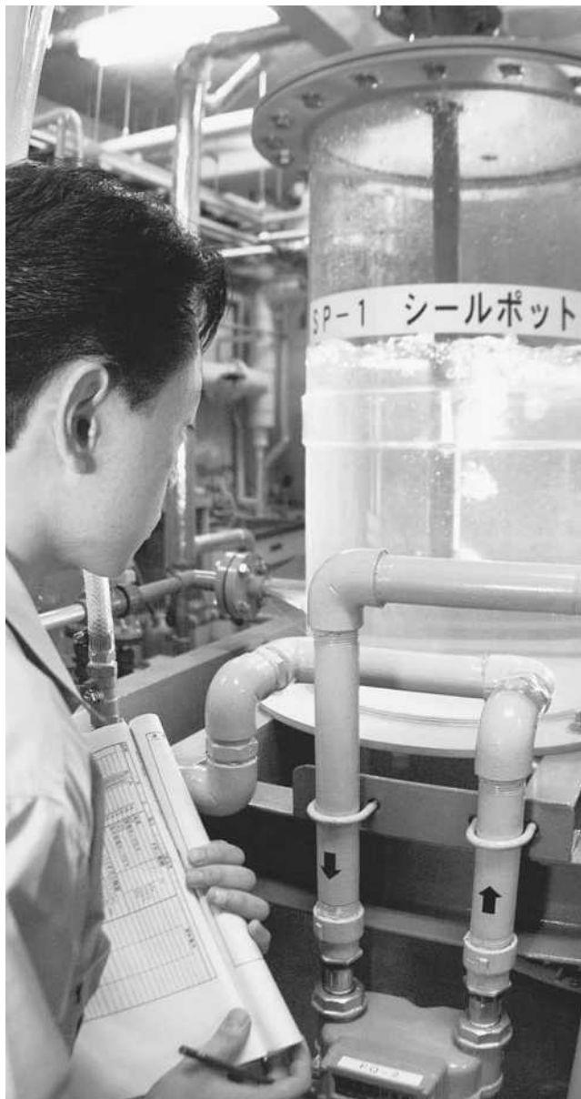
A researcher checks a sealed pot of methane in Kajima Corp.'s newly developed system designed to break down organic waste. (Corbis-Bettmann)
