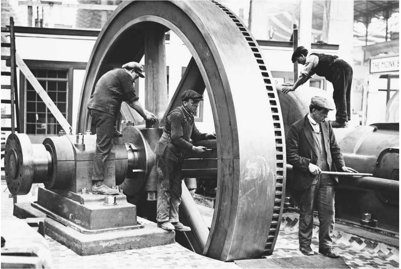
A 23-ton flywheel in the Palace of Engineering at the 1924 British Empire Exhibition. (Corbis Corporation)
