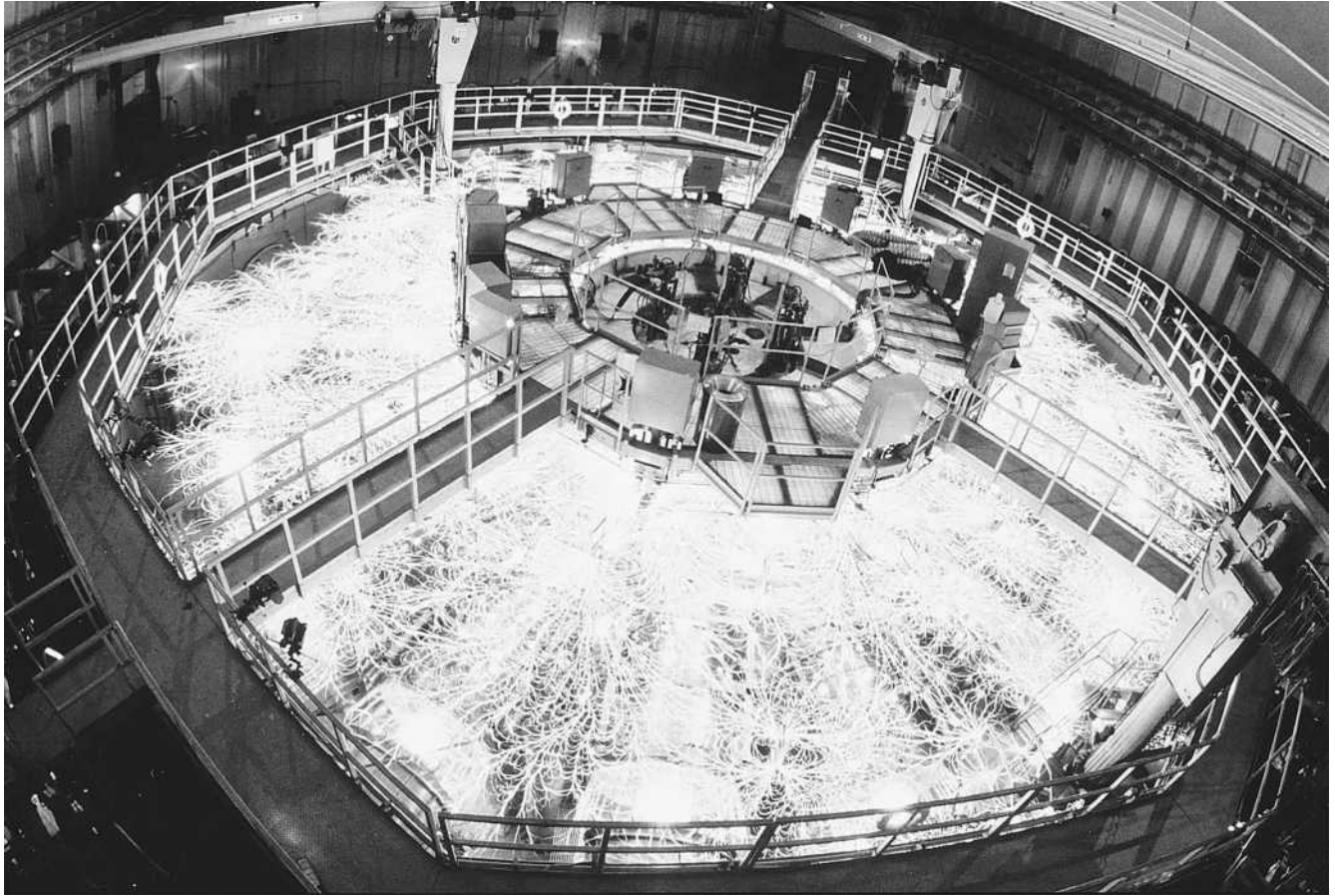
Particle beam fusion accelerator II (PBFA-II) was designed to deliver at least 100 trillion watts of power and was the first machine with the potential to ignite a controlled laboratory fusion reaction. (U.S. Department of Energy)
