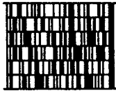
Fig. 10.7.6 Code 49. ( Uniform Symbology Specification Code 49, Copyright© 1993 Automatic Identification Manufacturers, Inc. )
