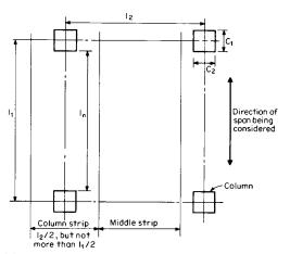
Fig. 12.3.11 Arrangement of typical slab panel.
