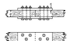
Fig. 12.2.17 Bolted splices for timber framing.
