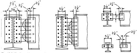
Fig. 12.2.19 Framed beam connections.
