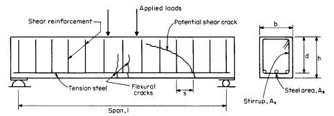
Fig. 12.3.1 Typical arrangement of reinforcement in beams.
