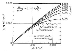
Fig. 12.3.6 Design factors for single reinforced concrete beams.
