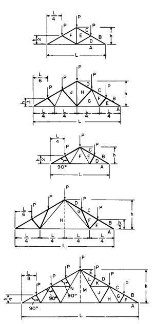
Fig. 12.2.2 to 12.2.6 Types of steep roof trusses.
