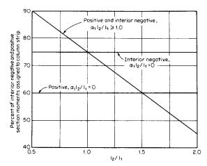
Fig. 12.3.13 Percentage of interior negative and positive moments assigned to a column strip.
