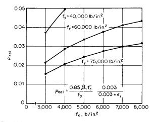
**Fig. 12.3.3** Balanced steel ratio as a function of  $f_v$  and  $f'_c$ .
