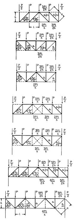
Fig. 12.2.7 to 12.2.13 Types of floor and roof trusses.
