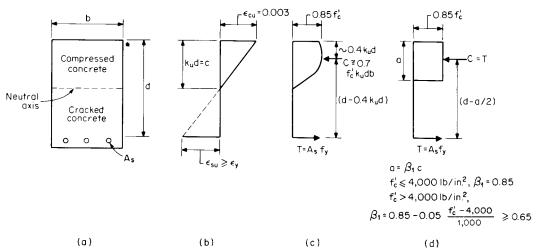
Fig. 12.3.2 Stress and strain distribution in reinforced concrete beam at failure. (*a*) Section; (*b*) strains; (*c*) stresses; (*d*) approximate stresses.
