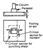
Fig. 12.3.14 Two-way reinforced concrete footing.
