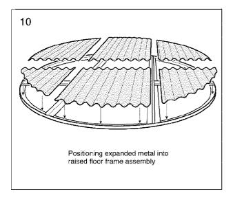
**10.** Some sections of corrugated expanded metal can be dropped into the corresponding frame sections. The last section can now be added while standing on top of the corrugated expanded metals and bolted in. The final section of corrugated expanded metal can now be positioned to complete the raised floor assembly.
