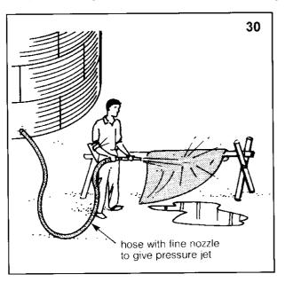
from filter fabric. Roll up fabric strips and remove all four layers from tank. Treat fabric with care and it will last for a long time.
