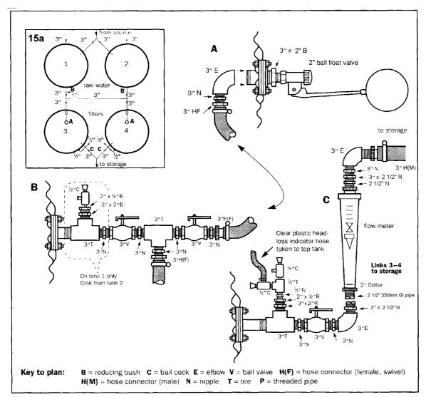
**15.** It is strongly recommended that all hoses and fittings are laid out following the plan before starting to make any connections, so that the correct layout and use of fittings is ensured.
