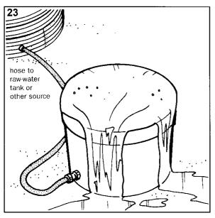
23. Ensure that excess water will drain away from the tanks. Fill drum to the brim with sand and level off. Slowly open valve at the tank outlet to allow water to flow into the drum, fluidise the sand, and so carry the silt upwards and away in the overflow. Open valve fully and allow to flow for about five minutes, or until overflow appears clear. If a large proportion of original sand has been removed, top up and wash again, in order to conserve water.
