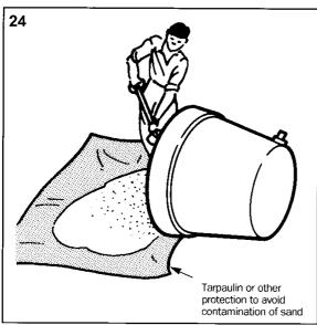
**24.** Disconnect hose from drum and allow water to drain out. Shovel the first half of clean sand out of the drum and tip the remainder out. Avoid contact between the clean sand and the ground (tarpaulin provided).
