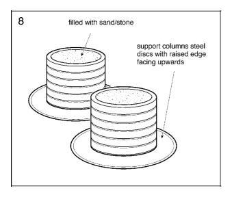
**8.** The columns are positioned on base plates (steel discs) with the raised edge facing upwards. This helps distribute weight and protect the liner. The columns should be filled to the brim with sand/stone to give additional strength to the structure.
