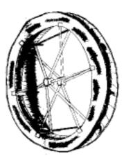
The wheels above are made of spokes of 12 mm round iron and pieces of 1" pipe, which are cut in half and welded at the end of the spoke.
