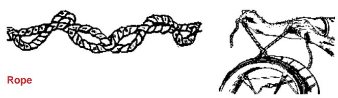
In Nicaragua an approximately 5 millimetres diameter polypropylene fibre rope is used. The rope, together with the pistons, functions as an endless band transporting water. The pistons are located the entire length of the rope and are attached with two knots, one in front of the piston and one directly behind it.
