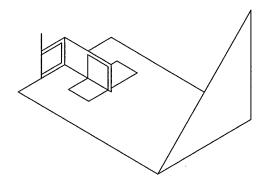
push hard on the prop; it will distort the blade. If the gage is on a board, you can add a little piece of masking tape to the blade to weight it and tilt the gage so the wire is nearly horizontal. The blade should drop onto the angle. If both the leading and trailing edges touch the angle, the pitch is set correctly. If not, the hub needs some twisting.
