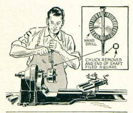
small work, this simple speed wrench will save considerable time. It is nothing more than an ordinary hand drill with the chuck removed and the end of the shaft squared to fit the chuck screws.
