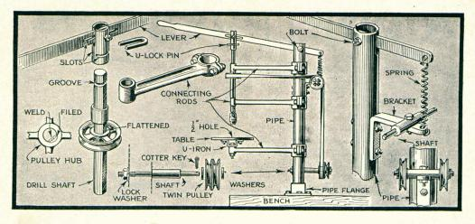
direct to the motor. In either case it is advisable to use a three-step pulley on the motor to provide speed adjustment. Accessories such as the V-pulleys, belts and chuck can be obtained from almost any dealer of home workshop supplies.
