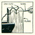
Wishing to save wire removed from hay bales for future use, a farmer straightened it by pulling it through slots cut in the end of a hardwood plank as shown. The
