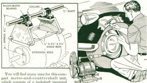
You will find many uses for this compact motor-and-countershaft unit, which consists of a jackshaft mounted on an electric motor. The unit can be fastened in a fixed position for driving power tools, such as metal-turning lathes, drill presses, etc., where various speeds are required, or it can be carried about for operating a flexible shaft as shown. By using two 5-in. cone pulleys and a motor of 1,750 r.p.m. on the original unit a speed range of 700 to 4,375 r.p.m. was obtained.
