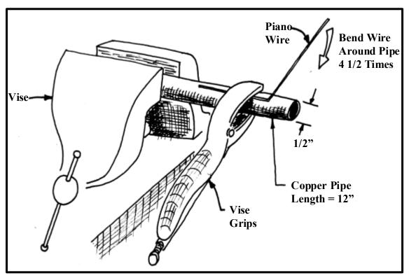
Figure 3 Coil Winding Setup
