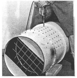
Holes in side of drum should be drilled with 1/2-in. bit in 3/8-in. slow-speed drill. To locate them, tape paper pattern over the drum
