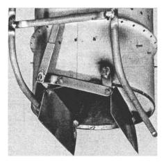
When brazing the ash doors to their 1/2-in. conduit pivots, support them horizontally on insulation bricks piled on the grate. These bricks won't conduct the heat
