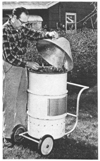
The burner may be used anywhere on your lawn without damaging the grass. When the 7-in. ash dump in the bottom is full, you merely wheel the cart to the trash heap and dump it with the flip of a lever
