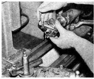
Employing the center mark that's etched on the slide and the plastic or steel scale, set off desired amount of offset with an Allen wrench.
