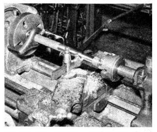
This adjustable offset-center attachment fits the tailstock ram. Turn the taper exactly the same as if tailstock had been set off center conventionally.
