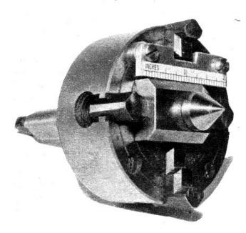
A small four-jaw chuck is the principal component of this gadget. Replace the No. 1 Morse-taper shank with a No. 2 shank. Make the sliding member from machine steel. Pin or cement a 2-in. length of plastic or steel rule to a metal plate and screw the plate to the chuck as shown. Use the headstock center as a guide when lining up the scale's center mark. To keep the slide parallel to the lathe bed, scratch a mark on the tailstock ram and a matching mark on the back of the chuck.
