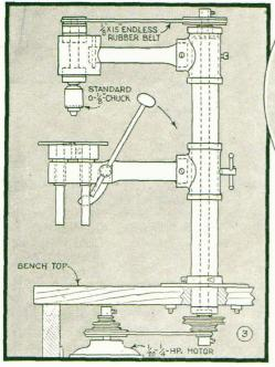
pieces of steel, brass and flat iron. Any small utility or sewing-machine motor will do to drive the press, although it is advisable to use a motor of the induction type having end thrust bearings, if it is to be mounted in a vertical position beneath the bench as shown. From Fig. 3 you can get a general idea of how the parts fit together, and how the chuck and motor are belted to a central jackshaft enclosed in the col-
