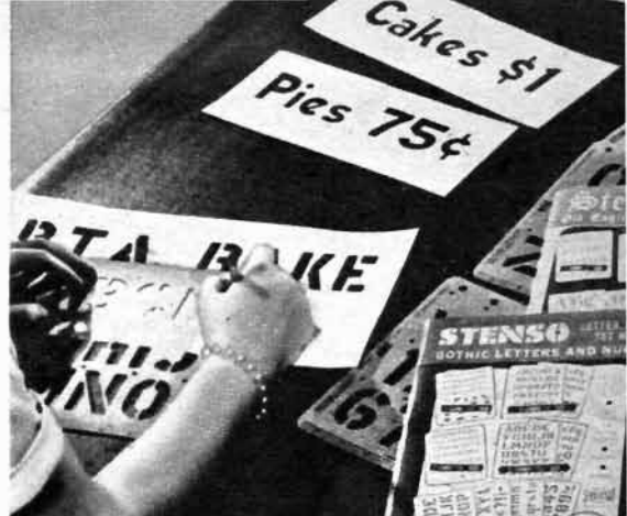
9. Stencil lettering guides come in Roman, Gothic and Old English letters, in sizes \frac{1}{2} to 2 \frac{1}{2} in.; they can be used many times.
