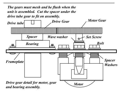
the drive unit must now be checked. Hook the battery cables to a 12 volt battery, red clip to positive. When you turn the power switch on the motor should run. Looking at the drive tube gear it should be turning counterclockwise. If it is not, double check your wiring. If the motor is not running turn the rheostat fully clockwise. If the wiring is correct and the motor is running backwards then the motor magnets are reversed.
