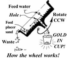
In this article we are only discussing building a machine with at least 7 spirals and which has a center hole which goes all the way through the wheel. An active water spray system is also necessary for accurate separation.
