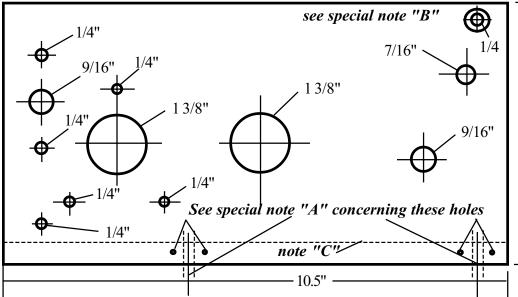
Special Notes: "A" Drill two 3/32" holes at each location and re-inforce doubler with two #8 sheet metal screws..Drill two 5.5" #7 holes (.201") from bottom, tap these 1/4-20.
