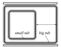
The small tub is at least 6" shorter and not as wide as the big tub... If the big tub is 14" wide and 22" long the little tub should not be larger than 12" x 16". Big tub should be 12" deep, small one 6" deep.
