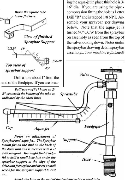
Attach the hose to the end of the feedpipe using a vinyl tube bushing or wrap electrical tape around the feedpipe to make it a slightly larger size than the I.D. of the feed hose. Push the feedhose firmly onto the feedpipe.
