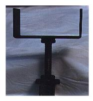
This stand can be used when cutting long lengths of material on a power hacksaw, chop sway, portable band saw, cold saw, etc. Two stands can be used adjustable sawhorses to support material during welding,
