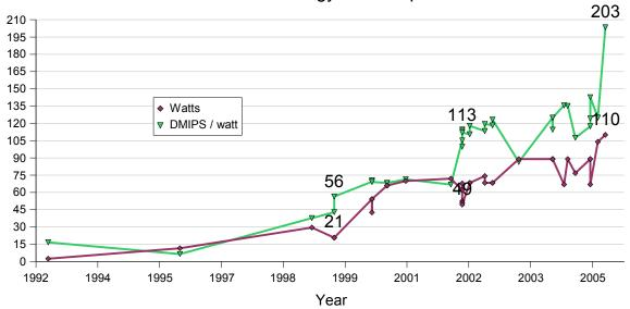
Although AMD CPUs weren't very efficient before 2002, their move to Silicon on Insulator (SOI) manufacturing and their focus on performance per watt and per clock cycle has made them more efficient than Intel CPUs for desktop computers. AMD's Dhyrstone MIPS per watt is rising rapidly while the wattage has risen more slowly.
