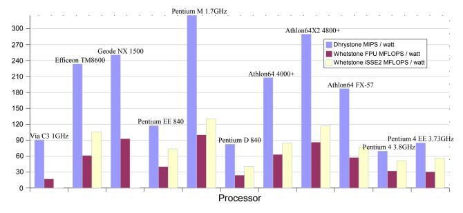
On the desktop, Athlon 64 chips are significantly more efficient than Pentium D and Extreme Edition, but the most efficient CPUs are mobile chips such as the Pentium M and Turion MT. Low powered options like the Efficeon and Core Solo are also not bad choices.
