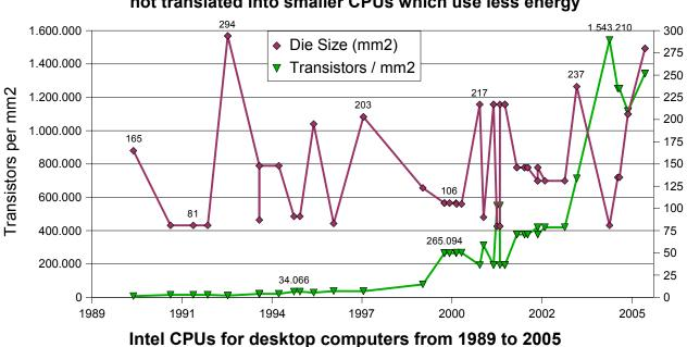
Advances in minaturization and transistor density have not translated into smaller CPUs which use less energy
