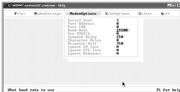
Figure 8-1: Configuring the modem in ToneLoc's TLCFG utility.
