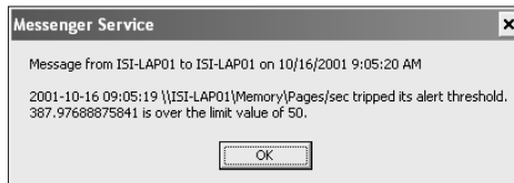
Figure 14-3: An alert message stating that lots of disk paging is going on.
