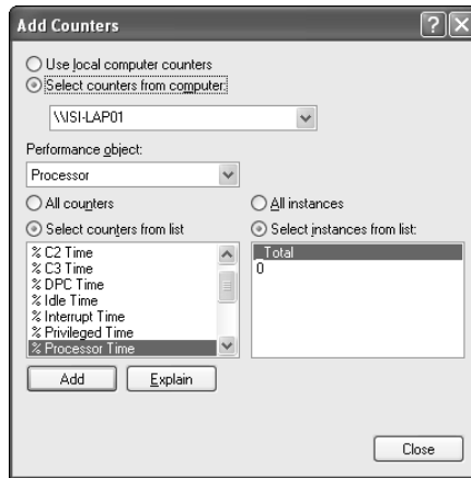
Figure 14-1: Adding a counter to an object in the Performance console's System Monitor.
