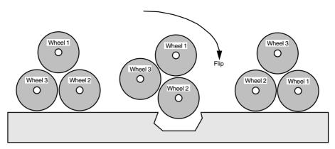
FIGURE 23.9 How the wheel gang "flips" when it encounters a hole or obstacle. The same basic motion can be used to climb stairs.
