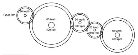
**FIGURE 17.7** Gears driven by the 20-tooth gear on the left rotate at different speeds, depending on their diameter.
