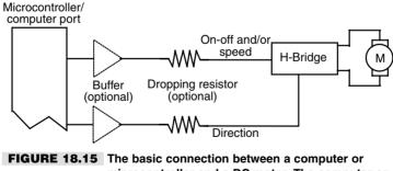
FIGURE 18.15 The basic connection between a computer or microcontroller and a DC motor. The computer or microcontroller operates the on/off control and the speed of the motor.
