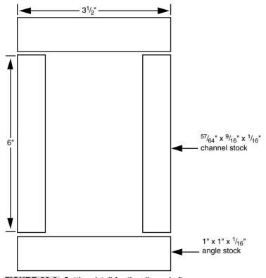
FIGURE 26.6 Cutting detail for the elbow shaft.
