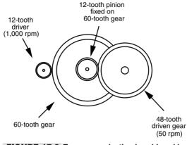
FIGURE 17.8 True gear reduction is achieved by ganging gears on the same shaft.
