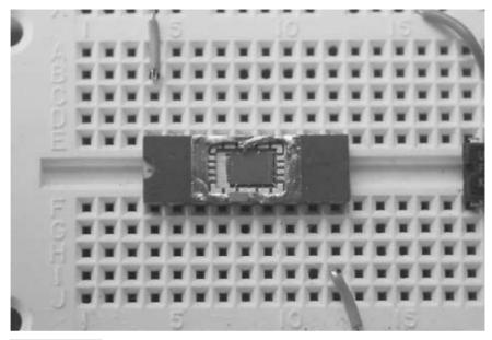
FIGURE 37.8 A static RAM chip with its lid removed. Once the lid is off, the semiconductor die inside can see the light of day, and any other light for that matter.
