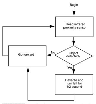
FIGURE 7.1 Use a flowchart to map out the functionality of your robot control programs.
