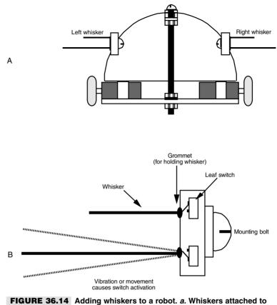
the dome of the Minibot (see Chap. 8); *b*. Construction detail of the whiskers and actuation switches.
