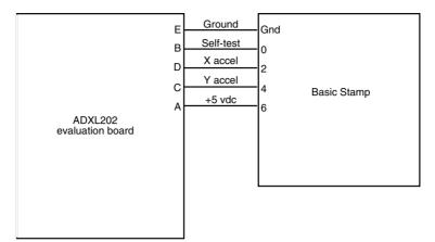
FIGURE 41.6 Connection diagram for hooking up an ADXL202EB (Evaluation Board) to a Basic Stamp II microcontroller.
