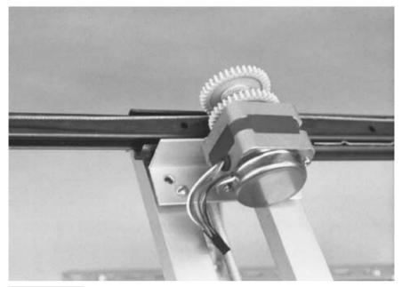
FIGURE 26.10 The rail motor mounted in place.
