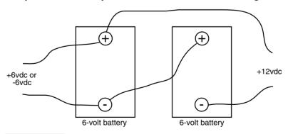
FIGURE 15.7 Various voltage tap-offs from two 6-volt batteries. This is not an ideal approach (the batteries will discharge at different rates), but it works in a pinch.
