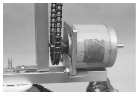
FIGURE 26.8 Mounted elbow motor with chain sprocket and roller chain.
