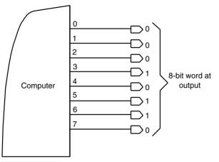
FIGURE 30.2 The parallel port outputs eight bits at a time.
