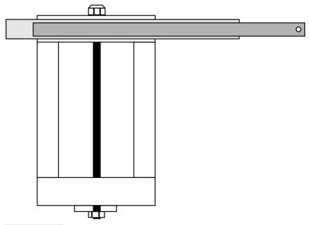
FIGURE 26.9 The recommended mounting location for the drawer rail.
