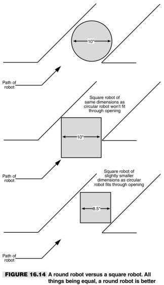
things being equal, a round robot is better able to navigate through small openings. However, rounded robots also have less usable surface area, so a square-shaped robot can be made smaller and still support the same onboard "real estate."
