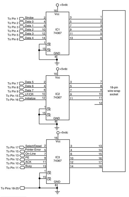
FIGURE 30.4 Schematic for the Robot Experimenter's Interface.
