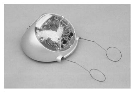
**FIGURE 36.13** The Movit WAO robot (one of the older models, but the newer ones are similar). Its two tentacles, or whiskers, allow it to navigate a space.
