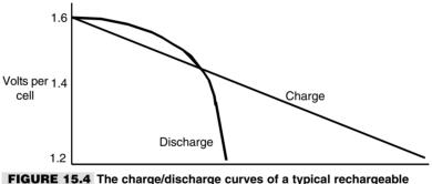
battery. Note that the charge time is longer than the discharge time.
