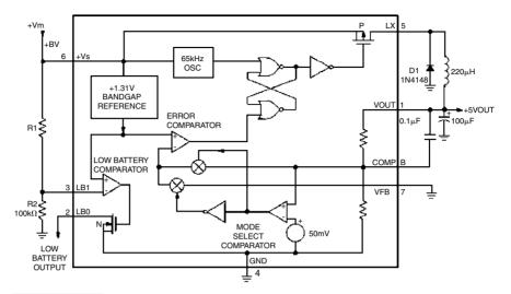
FIGURE 15.9 The Maxim MAX638 is among several high-efficiency voltage regulators available. The MAX638 is most commonly used to provide regulated +5 volts, but it can also be adjusted using external components to provide other voltages.
