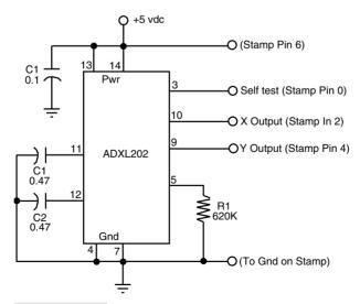
**FIGURE 41.5** Hookup diagram for the Analog Devices ADXL202 dual-axis accelerometer chip, with connections shown for a Basic Stamp II microcontroller.
