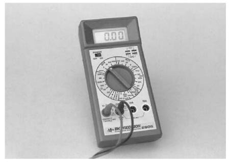
FIGURE 3.2 A volt-ohm meter (or multitester) checks resistance, voltage, and current. This model is digital and has a 3 1/2-digit liquid crystal display (LCD) readout.
