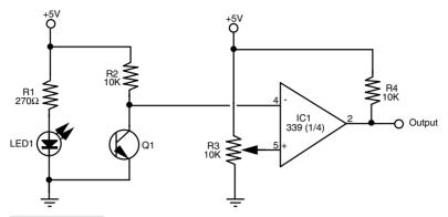
FIGURE 38.4 Connecting the LED and phototransistor to an LM339 quad comparator IC. The output of the comparator switches between HIGH and LOW depends on the amount of light falling on the phototransistor. Note the addition of the 10K "pullup" resistor on the output of the comparator. This is needed to assure proper HIGH/LOW action.
