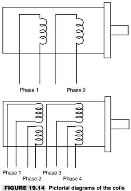
in a bipolar and unipolar stepper motor.
