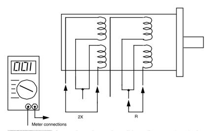
FIGURE 19.17 Connection points and possible readings on a 5- or 6-wire unipolar stepper motor.
