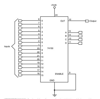
FIGURE 30.11 Basic wiring diagram for the 74150 multiplexer chip.
