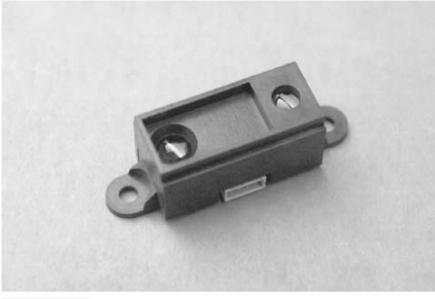
FIGURE 38.15 The Sharp infrared sensors are equipped with a focused infrared light source and a linear photodetector array. Distance can be determined by detecting where the reflected light touches the array.
