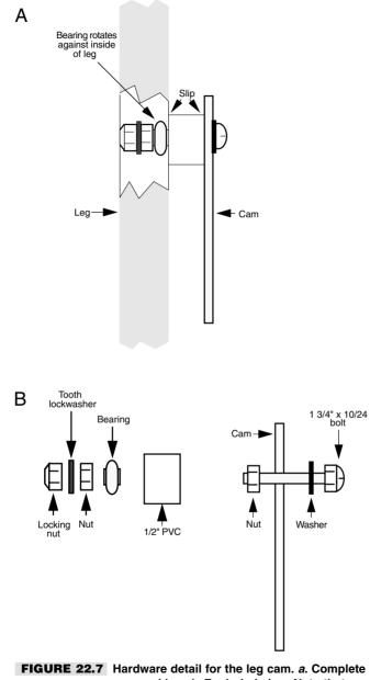
**IGURE 22.7** Hardware detail for the leg cam. *a*. Complete cam and leg; *b*. Exploded view. Note that two of the legs use a 2-inch piece of PVC and a 3-inch bolt.
