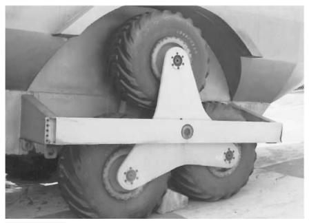
FIGURE 23.8 A close-up of the tri-star wheels used in the Landmaster.
