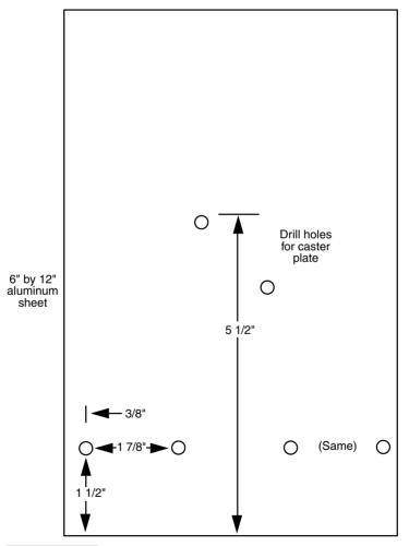
FIGURE 10.1 Drilling diagram for the Buggybot frame.
