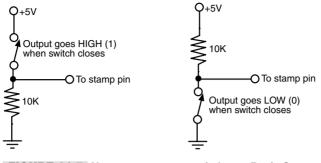
FIGURE 31.7 You can connect a switch to a Basic Stamp pin so that it triggers a 0 or a 1 state when it closes.
