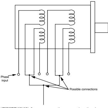
**FIGURE 19.16** Common connections may reduce the wire count of the stepper motor to five or six, instead of eight.
