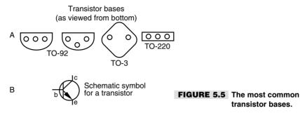
Transistors can be either NPN or PNP devices. This nomenclature refers to the sandwiching of semiconductor materials inside the device. You can't tell the difference between an NPN and PNP transistor just by looking at it. However, the difference is indicated in the catalog specifications sheet as well as schematically.
