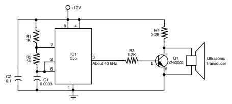
FIGURE 36.10 Schematic diagram for a basic ultrasonic proximity transmitter.
