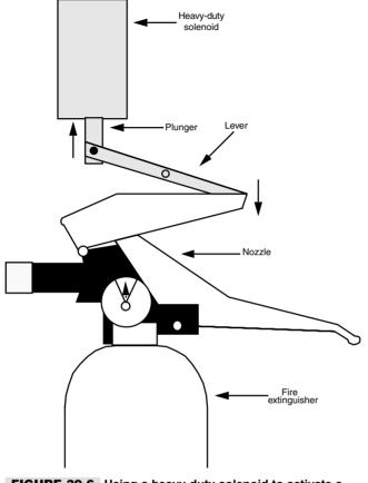
FIGURE 39.6 Using a heavy-duty solenoid to activate a fire extinguisher.
