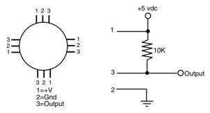
FIGURE 38.12 Circuit diagram for using the Dinsmore 1490 digital compass. When used with a +5 vdc supply, the four outputs can be connected directly to a microcontroller. One or two outputs can be activated at a time; if two are activated, the sensor is reading between the four compass points (e.g., N and W outputs denotes NW position).
