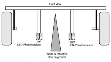
FIGURE 38.2 Placement of the left and right phototransistor-LED pair for the line-tracing robot.
