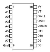
FIGURE 34.6 Pinout diagram for the Holtek HT-12D decoder.
