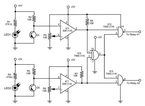
FIGURE 38.5 Wiring diagram for the line-tracing robot. The outputs of the 7400 are routed to the relays in Figure 38.6.
