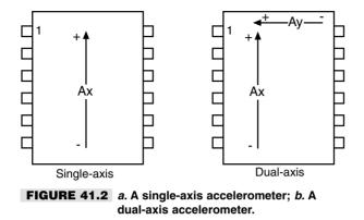
products. One of their key product lines is accelerometers, and for them they use a patented fabrication process to create a series of near-microscopic mechanical beams. This "micro-machining" involves etching material out of a substrate. During acceleration, the beam is distended along its length. This distention changes the capacitance in nearby plates. The change in capacitance is correlated as acceleration and deceleration.
