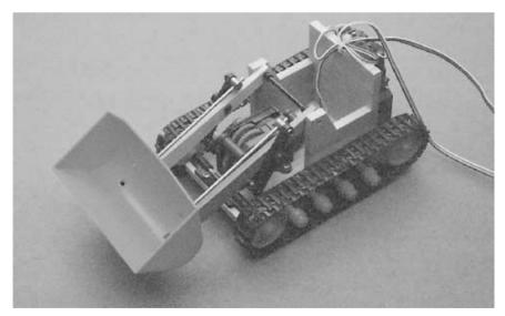
FIGURE 11.5 The Tamiya Bulldozer kit can be used as a lightweight robot platform. The kit comes with an interesting dual motor that operates the left and right treads.
