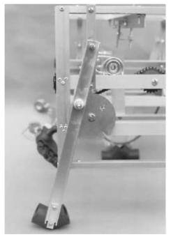
FIGURE 22.15 One of six legs, completed (shown already attached to the robot).
