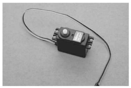
FIGURE 20.1 The typical radio-controlled (R/C) servo motor.
