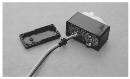
**FIGURE 20.2** The internals of an R/C servo. The servo consists of a motor, a gear train, a potentiometer, and a control circuit.
