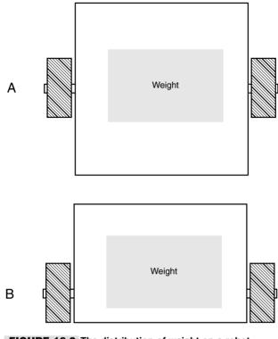
FIGURE 16.3 The distribution of weight on a robot affects its stability and traction. *a*. Centering the weight down the middle in a robot with two balancing casters; *b*. Sliding the center of balance toward the drive wheel in a single-caster 'bot.
