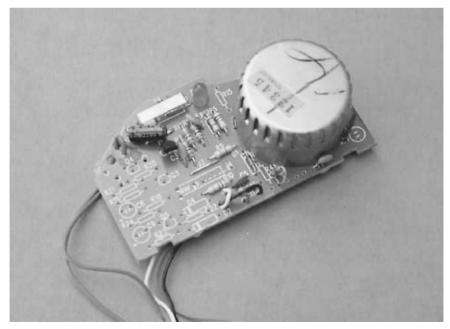
FIGURE 39.2 The guts of a smoke detector.
