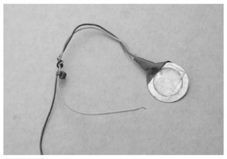
FIGURE 35.8 Piezo ceramic discs are ideally suited to be contact and pressure sensors for robotics.
