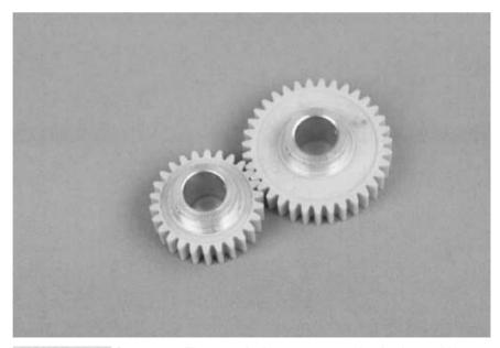
FIGURE 17.11 Spur gears. These particular gears are made of nylon and have aluminum hubs. It's better to use metal hubs in which the gear is secured to the shaft with a setscrew.
