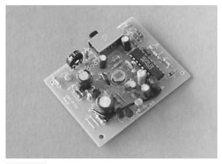
FIGURE 36.8 A hacked PIR detector, showing the DC-operated circuit board.
