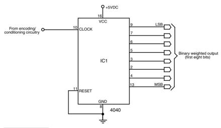
FIGURE 18.17 The basic wiring diagram of the 4040 CMOS 12-stage ripple counter IC.
