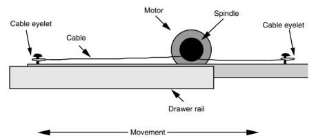
FIGURE 26.12 Threading detail for the drawer cable assembly.
