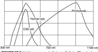
FIGURE 37.2 Light sensors vary in their sensitivity to different colors of the electromagnetic spectrum. The color sensitivity of CdS cells is very similar to that of the human eye.
