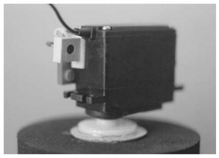
**FIGURE 20.10** For greater control and accuracy, use an external 5K or 10K pot to replace the one removed from the servo.
