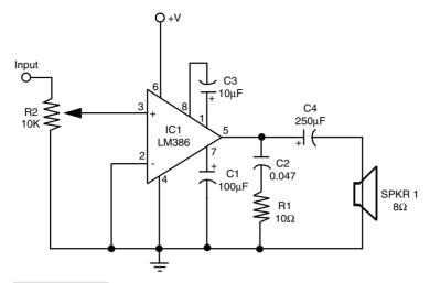
FIGURE 40.7 A simple gain-of-200 integrated amplifier.
