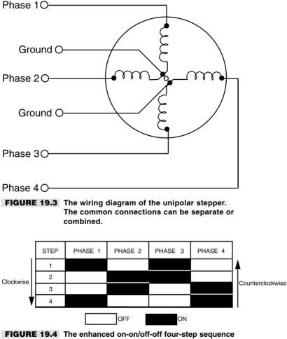
of a unipolar stepper motor.
