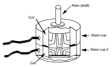
FIGURE 19.2 Inside a unipolar stepper motor. Note the two sets of coils and stators. The unipolar stepper is really two motors sandwiched together.
