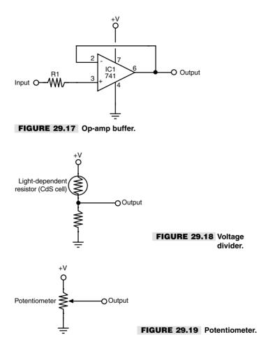
Like a phototransistor, the output of a *photodiode* is a varying current. This output can also be converted into a voltage by using a resistor (see Fig. 29.18). (The higher the resistance, the higher the sensitivity of the device.) This output tends to be fairly weak—on the order of millivolts instead of volts. Therefore, amplification is usually required.
