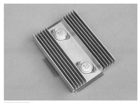
FIGURE 18.7 Power transistors mounted on a heat sink.
