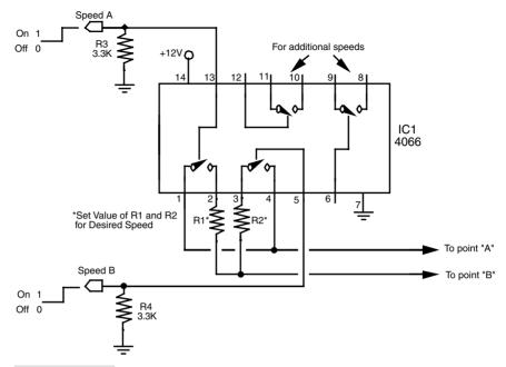
**FIGURE 18.14** Using a 4066 CMOS analog switch to remotely control the speed of the motor. Use a device such as the 4051 for even more speed choices.
