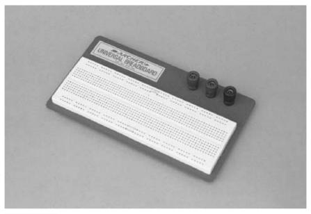
FIGURE 3.4 Solderless breadboards are used to "try out" a circuit before soldering. Some robot makers even use them in their final prototypes.
