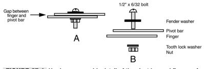
FIGURE 27.4 Hardware assembly detail of the pivot bar and fingers of the two-pincher gripper. *a*. Assembled sliding joint; *b*. Exploded view.
