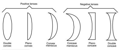
FIGURE 37.10 Lenses come in a variety of forms. Plano-convex and double-convex are among the most common.
