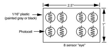
FIGURE 37.6 Mounting the photocells for an eight-cell eye.
