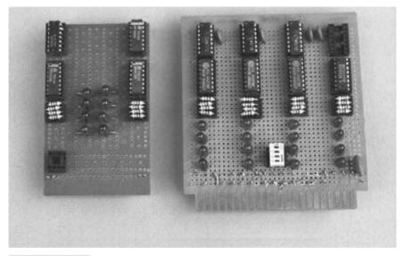
FIGURE 19.12 Two finished stepper motor translator boards, with indicator LEDs. The board on the left controls two stepper motors; the board on the right controls four stepper motors.
