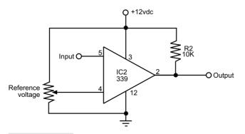
FIGURE 29.15 Voltage comparator input.
