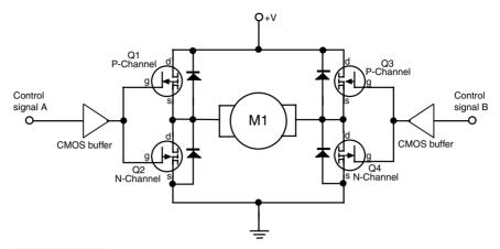
FIGURE 18.9 Combination N- and P-channel MOSFET transistors can be used to increase the voltage flowing to the motors. The MOSFETs should be "complementary pairs" (made to work with one another) that share the same voltage and current ratings. Most makers of MOSFET transistors provide complementary N- and P-channel products.
