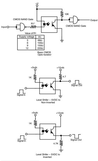
FIGURE GROUP D.4. Opto-isolator interfacing.
