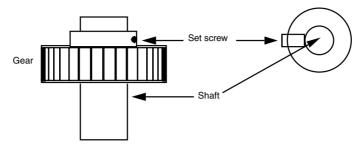
FIGURE 17.15 Use a setscrew to secure the gear to the shaft.
