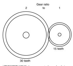
FIGURE 17.6 A representation of a 2:1 gear reduction ratio.
