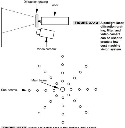
FIGURE 37.14 When projected onto a flat surface, the beams from the diffracted laser light form a regular grid.
