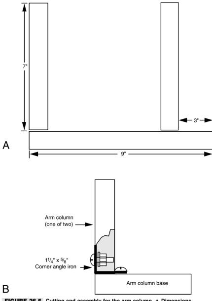
**FIGURE 26.5** Cutting and assembly for the arm column. *a.* Dimensions of pieces; *b.* Hardware assembly detail.
