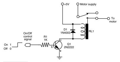
FIGURE 18.2 Using a relay to turn a motor on and off. The input signal is TTL/microprocessor compatible.
