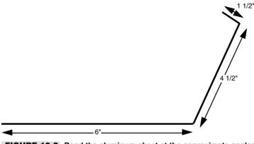
FIGURE 10.2 Bend the aluminum sheet at the approximate angles shown here.
