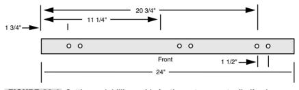
FIGURE 22.4 Cutting and drilling guide for the motor mount rails (four).
