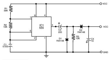
FIGURE 15.12 A polarity inverter circuit. Current output is low but enough for a few op amps.
