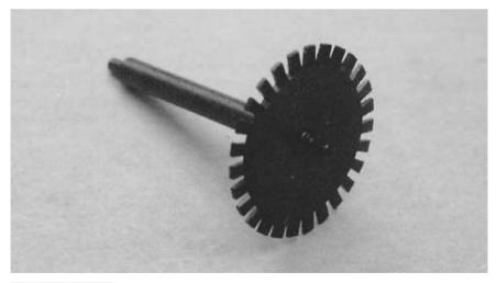
FIGURE 18.20 The typical PC mouse contains two shaft encoder discs. They are about perfect for the average small-or-medium-size robot.
