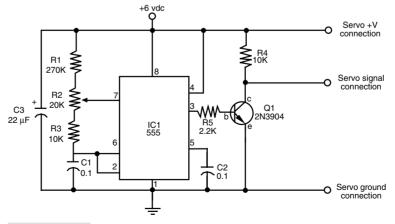
FIGURE 20.7 A 555 timer IC can be used to provide a control signal to a servo.
