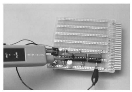
FIGURE 3.3 The logic probe in use. The probe derives its power from the circuit under test.
