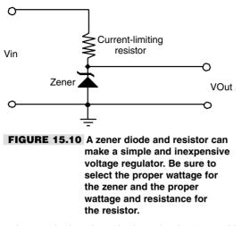
resistor R1 in the schematic shown in Fig. 15.10. This resistor limits the current through the zener, and its value (and wattage) is determined by the current draw from the load, as well as the input and output voltages.
