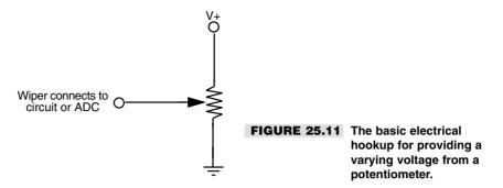
ter may provide a relative measurement of the position of the arm, but the information is in analog form, as a resistance or voltage, neither of which can be directly interpreted by a computer.
