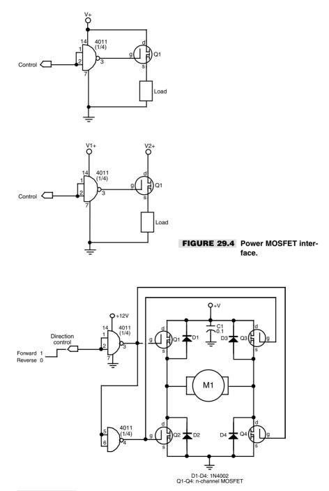
FIGURE 29.5 Discrete component H-bridge interface.
