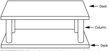
FIGURE 16.1 "Decked" robots provide extra space for batteries and electronics, but they can also add considerably to the weight. Use lightweight construction materials to avoid unduly increasing the weight of the robot.
