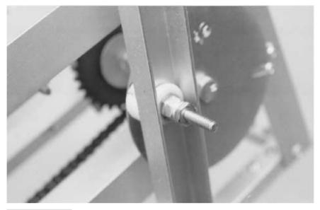
FIGURE 22.16 A close-up detail of the leg cam.
