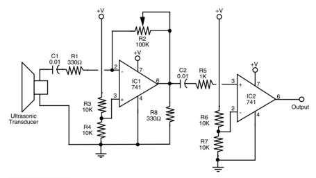
FIGURE 36.11 Schematic diagram for a basic ultrasonic proximity receiver.
