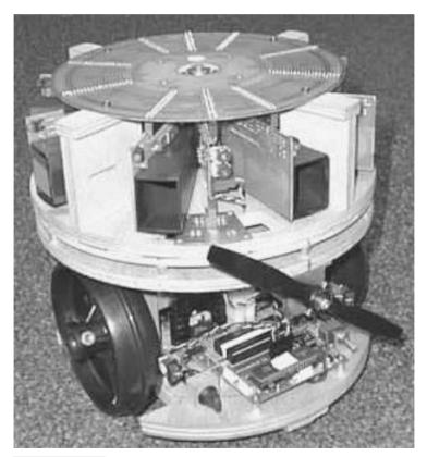
FIGURE 33.2 This fire-fighting robot, built by OOPic developer Scott Savage, uses three OOPics wired together in a network to control the machine's central command, sensors, and locomotion.
