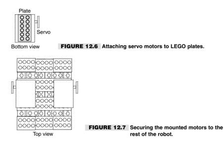
straight, and make sure the plate doesn't block the seam in the case of the servo (this will make it easier to disassemble the servo, if you need to for whatever reason).
