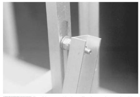
**FIGURE 22.13** The slider cam and hardware. The slot must be smooth and free of burrs, or the leg will snag.
