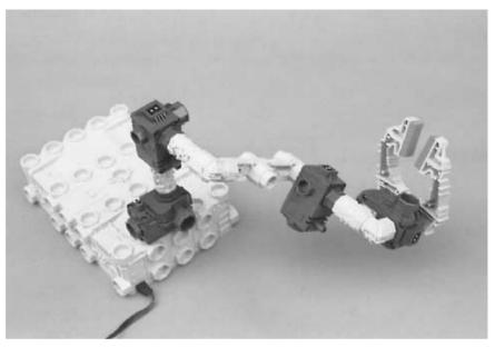
FIGURE 11.2 The robot arm constructed with parts from a Robotix construction kit.
