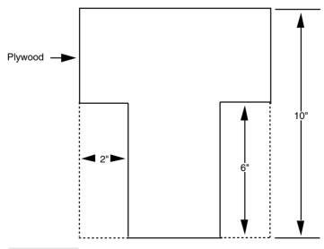
**FIGURE 9.1** Cutting plan for a square plywood base.
