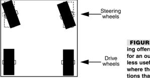
**FIGURE 16.11** Car-type steering offers a workable alternative for an outdoors robot, but it is less useful indoors or in places where there are many obstructions that must be steered around.
