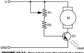
FIGURE 18.11 How not to vary the speed of a motor. This approach is very inefficient.
