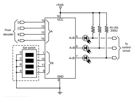
**FIGURE 18.19** The basic wiring diagram of a single-state magnitude comparator circuit.
