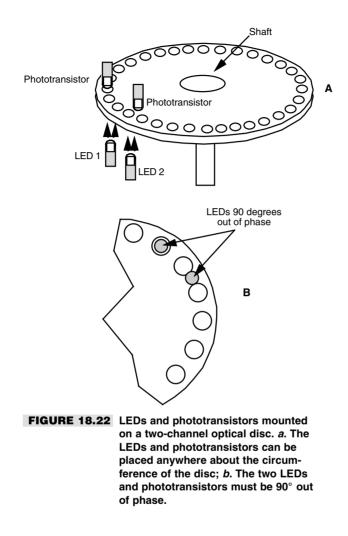
slip. You can determine if the wheels are moving when they aren't supposed to be, and you can determine the direction of travel. This so-called two-channel system uses *quadrature encoding*—the channels are out of phase by  $90^{\circ}$  (one quarter of a circle).
