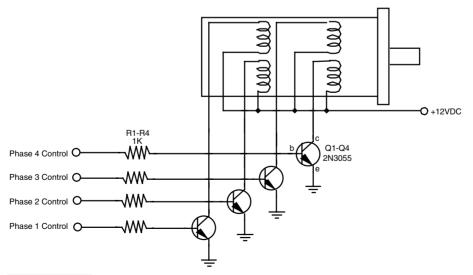
**FIGURE 19.6** The basic hookup connection to drive a stepper motor from a computer or other electronic interface. The phasing sequence is provided by software or other means through a port following a four-bit binary sequence: 1010, 0110, 0101, 1001 (reverse the sequence to reverse the motor).
