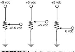
FIGURE 20.4 A potentiometer is often used as a variable voltage divider. As the potentiometer turns, its wiper travels the length of a resistive element. The output of the potentiometer is a varying voltage, from 0 to the +V of the circuit. Therefore, when experimenting with servomotors exercise care to avoid pushing them beyond their natural limits.
