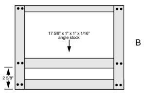
FIGURE 22.5 The motor mount rails secured to the robot. *a*. The long rail mounts 2 1/2 inches from the bottom of the frame (the holes drilled earlier point up); *b*. The short end crosspiece rail mounts 2 5/8 inches from the bottom of the frame.
