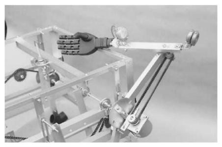
FIGURE 22.26 An arm attached to the front side of the Walkerbot.
