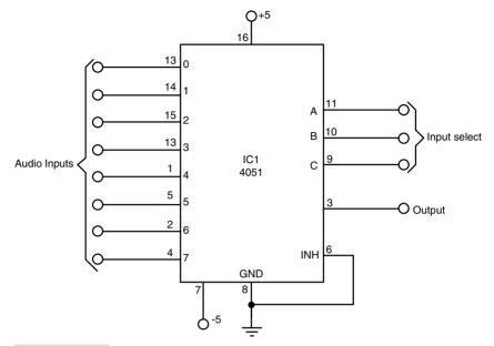
**FIGURE 40.5** How to use the 4051 CMOS 8-input analog switch to control the output of the various sound-making circuits in your robot. You can choose the sound source you want routed to the output amplifier by selecting its input with the Input Select lines (they are binary weighted: A = 1, V = 2, C = 4). For best results, the audio inputs should not already be amplified.
