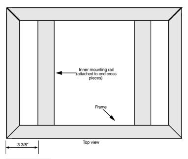
FIGURE 22.18 Mounting location of the inner rails.
