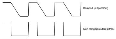
FIGURE 13.6 The RCX uses pulse-width modulation to vary the power level of its three outputs. The pulses can be steep square waves, or they can be ramped.
