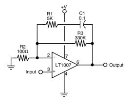
FIGURE 40.2 Preamplifier circuit for use with a magnetic tape playback head.
