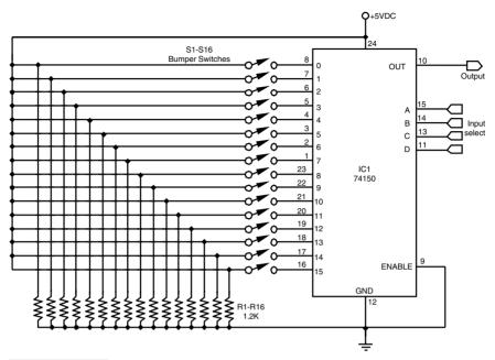
FIGURE 36.17 Multiple switch detection using a 74150 multiplexer IC.
