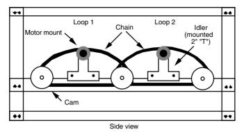
FIGURE 22.21 Mounting locations for idler sprocket.
