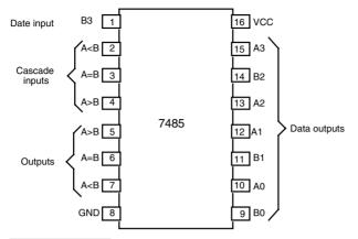
FIGURE 18.18 Pinout diagram of the 7485 magnitude comparator IC.
