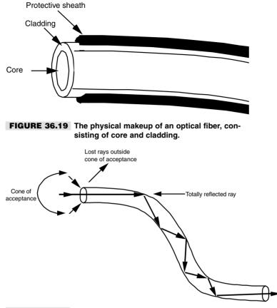
FIGURE 36.20 Light travels through optical fibers due to a process called total internal reflection (TIR).
