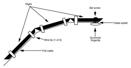
FIGURE 27.17 A design for an experimental compliant finger. Make the finger spring-loaded by attaching a spring to the back of the finger (a strip of lightweight spring metal also works).
