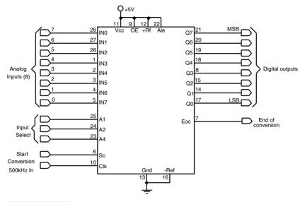
FIGURE 29.20 Basic hookup circuit for the ADC0809 analog-to-digital converter.
