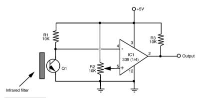
FIGURE 39.1 A flame detector built around the LM399 quad comparator IC.
