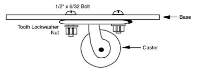
FIGURE 10.6 Mounting the caster to the Buggybot.
