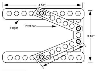
FIGURE 27.3 Construction detail of the basic two-pincher gripper, made with Erector set parts.
