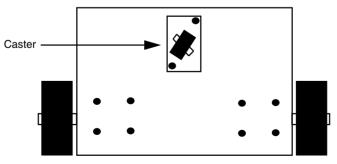
FIGURE 16.6 A robot with a front-drive motor mount uses a single opposing caster for balance. Steering is accomplished using the same technique as a centerline motor mount.
