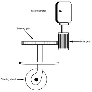
FIGURE 23.5 The steering gear up close.
