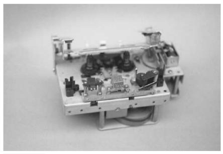
FIGURE 40.1 A surplus cassette deck transport. This model is entirely solenoid driven and so is perfect for robotics.
