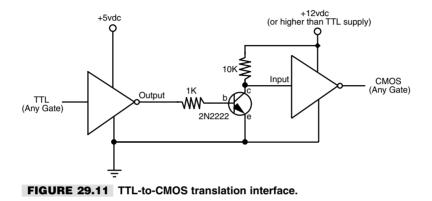
Fig. 29.11 shows how to interface TTL (5 volt) to CMOS circuits that use different power sources (use this circuit even if both circuits run under +5 vdc). Fig. 29.12 shows the same concept, but for translating CMOS circuits to TTL circuits that use different power sources.
