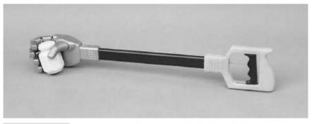
FIGURE 27.16 Commercially available plastic robotic arm and hand toy. The gripper can be salvaged for use in your own designs. The opposing thumb is not articulated, but the fingers have a semi-compliant grip.
