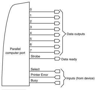
FIGURE 30.3 The minimum parallel port: eight data outputs, a STROBE (Data Ready) line, and inputs from the printer, including Select, Printer Error, and Busy.
