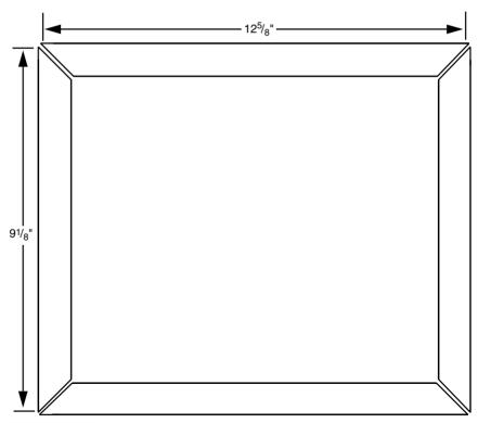
FIGURE 21.1 Cutting diagram for the Roverbot.
