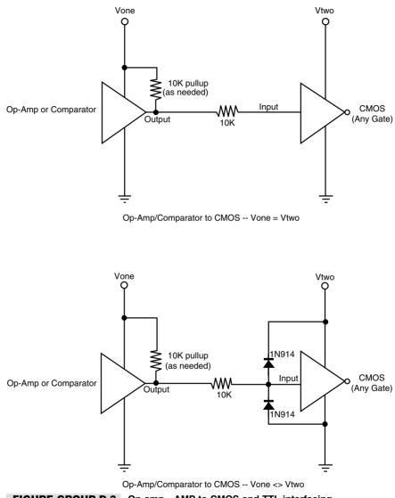
FIGURE GROUP D.3. Op-amp—AMP to CMOS and TTL interfacing.
