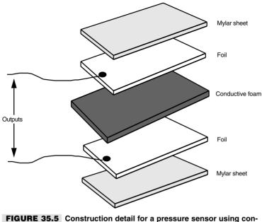
FIGURE 35.5 Construction detail for a pressure sensor using conductive foam. The leads are soldered or attached to foil (copper works best). Choose a foam that has a good "spring" to it.
