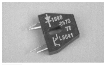
FIGURE 36.3 The Texas Instruments TIL139 infrared emitter/detector sensor unit. These types of units are often available on the surplus market.
