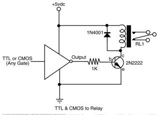
FIGURE GROUP D.6. CMOS and TTL to RELAY and LED drivers.
