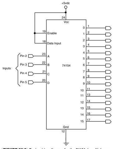
FIGURE 30.8 Basic wiring diagram for the 74154 demultiplexer chip.
