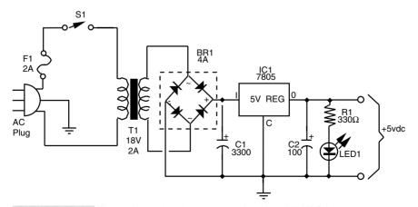
FIGURE 15.18 Five-volt regulated power supply using 117 VAC input.
