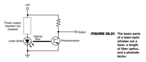
the relative intensity of the collision. The more the robot has "connected" to some object, the more the fibers will deform and the greater the output change of the light as it reaches the photodetector.
