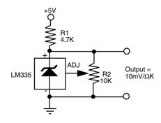
FIGURE 39.4 The basic wiring diagram for the LM355 temperature sensor.
