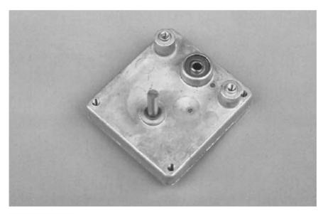
**FIGURE 17.10** A gear reduction box, originally removed from an open-frame AC motor. On this unit, the input and output shafts are on the same side.
