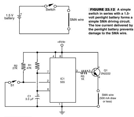
**FIGURE 23.13** A 555 timer IC is at the heart of an ideal driving circuit for SMA wire. The 555 removes the current shortly after you release activating switch S1.
