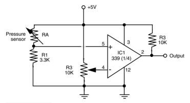
FIGURE 36.15 Converting the output of a conductive foam pressure sensor to an on/off type switch output.
