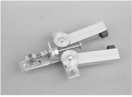
FIGURE 27.10 The finished two-pincher worm drive gripper.
