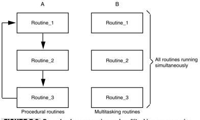
**FIGURE 7.2** Procedural programming and multitasking programming use subroutines in different ways.
