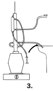
Now set the temperature at the column head. This is done by roughly setting the heat source and a fine adjustment of the cooling water. A perfect distillation takes place 1-2 tenths of a degree centigrade under boiling point of alcohol. Try to set 78°C. It is imperative that the temperature is under 80°C.
