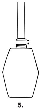
Undo the connector between the column and the boiling vessel and set aside the apparatus to cool. Air *must* be allowed into the vessel, otherwise the resultant vacuum can cause the boiling vessel to implode.
