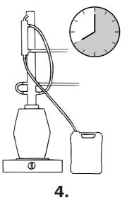
After 8-12 hours distillation (or other period of time) it is time to finish the process. Exactly when will be seen by the temperature at the column head. Either the temperature rises, so one switches off at 90°C. The temperature can also drop 10-20°C or more and the spirit stops dripping from the apparatus. This is because one has succeeded in setting the temperature so accurately and with the alcohol all gone from the mash the water cannot get through the
