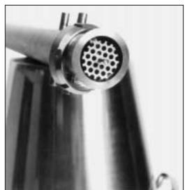
A small stainless strip is welded The perforated plate is across the base of the column, onto which is welded a small stainless steel set screw. The perforated plate is then attached holds the perforated plate, to this.
