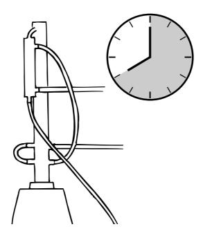
The principle of distillation is that one heats up the mash to boiling point and cools down the steam (condensation) to a liquid. Alcohol has a lower boiling point (78.3°C) than water (100°C) and so boils first. By this means the alcohol is separated from the mash.
