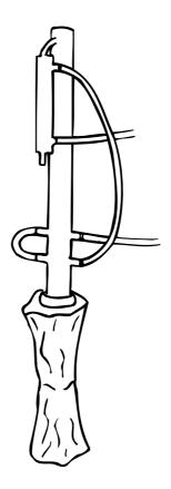
**Implosion** of the boiling vessel can occur. After distillation the mash cools in the boiling vessel and a vacuum forms. Air cannot get into the vessel through the column in time (the hose can also be twisted) so the boiling vessel shrinks like a rag.
