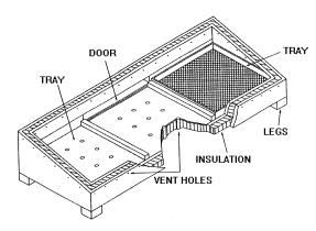
Figure 1: The solar cabinet drier
