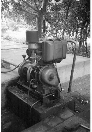
Figure 1: Diesel-driven pump ©ITDG
