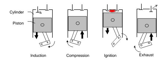
Figure 2. The four-stroke Diesel cycle
