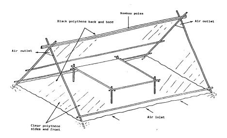
Figure 1: Typical Tent Solar Dryer
