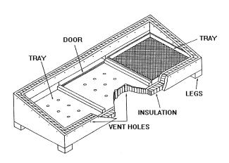
The Brace Solar Dryer as shown in Figure 2 has been widely used for small scale food drying. It consists of a wooden box with a hinged transparent lid. The inside is painted black and the food supported on a mesh tray above the dryer floor. Air flows into the chamber through holes in the front and exits from vents at the top of the back wall. Brace type dryers achieve higher temperatures, and thus shorter drying times, than tent dryers.
