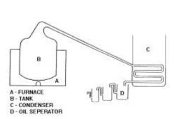
Figure 7: Distillation Equipment
