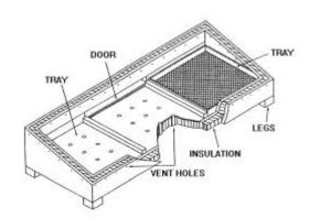
Figure 1: Solar Dryer
