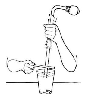
Figure 6: Tap the pipe to remove the mercury
