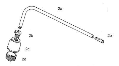
Figure 2: Part required for the retort
