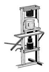
speed up removal of oil. The pressure should be increased slowly to allow time for the oil to escape. Screw types are more reliable than hydraulic types but are slower and produce less pressure. Except where a lorry jack is used (Figure 4), hydraulic types are more expensive, need more maintenance, and risk contaminating oil with poisonous hydraulic fluid.
