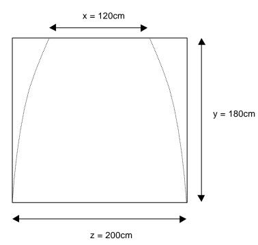
Figure 19: Dimensions for cutting sacking
