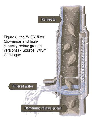
rudimentary. A German company, WISY, have developed an ingenious filter which fits into a vertical downpipe and acts as both filter and first-flush system. The filter, shown in Figure 8, cleverly takes in water through a very fine (~0.20mm) mesh while allowing silt and debris to continue down the pipe. The efficiency of the filter is over 90%. This filter is commonly used in European systems.
