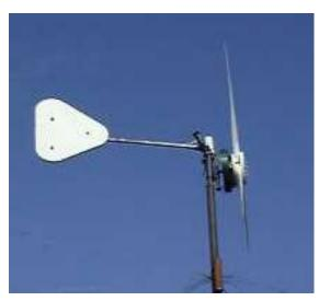
Figure 2: The ITDG wind generator for battery charging © ITDG
