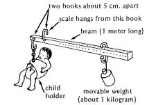
Weight is correct when beam stays horizontal.
