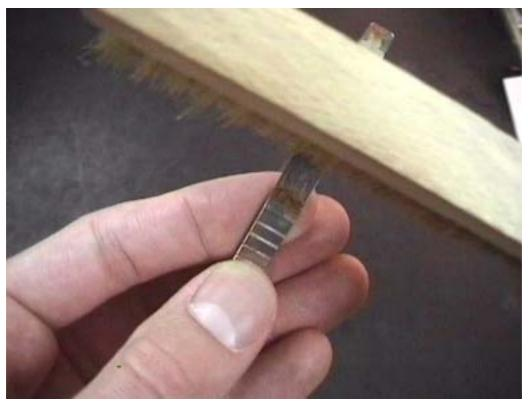
4. Do not use the brush on the working part of the instrument.
