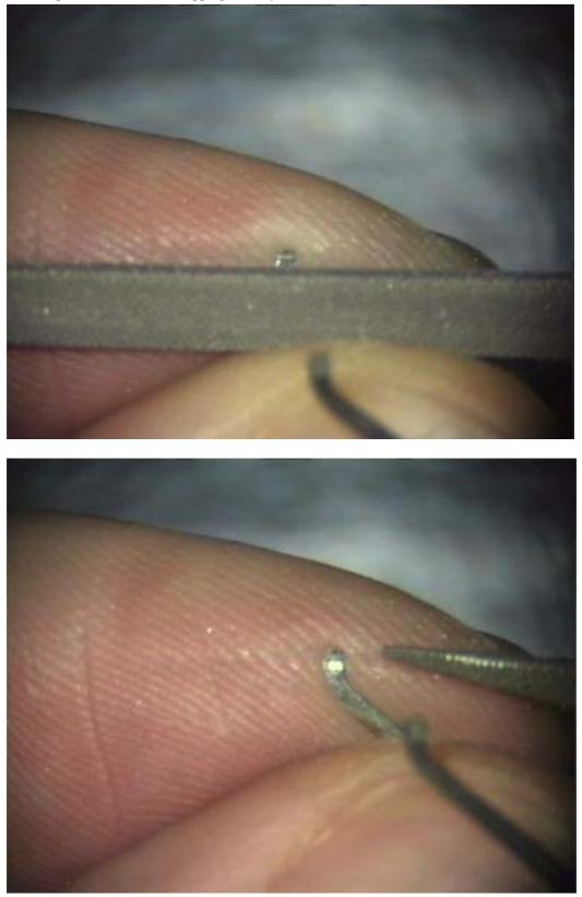
5. Make a groove on the other leg of the forceps at the same distance from the tip as on the first side.
