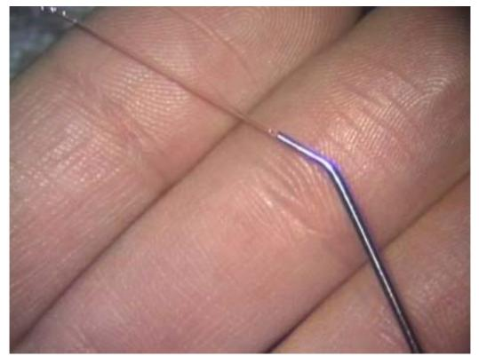
2. When cannula is blocked, use a small, fine piece of metal wire, to re-open the cannula. Use a soft type of metal wire, so the innerside of the cannula will not get scratched.
