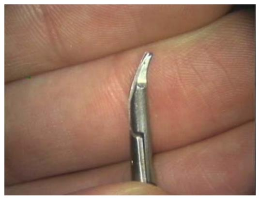
2. Rebend the bend side carefully, using a pair of flat tipped pliers. Do not use too much force.
