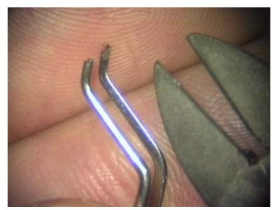
2. Smoothen both tips with a triangular file. Hold the tips of the forceps between thumb and index finger, this way the file cannot slip away.
