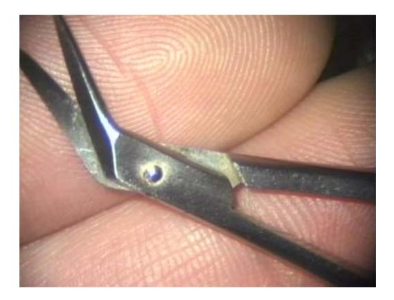
5. Open the lock of the instrument to make the joint accessible. Rotate the male part, so it can slip out of the female part. Do not use force to open the lock, since that might damage it.
