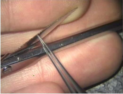
**2.** Enlargement of reflexion of a pit in cutting edge.
