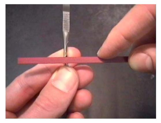
4. Sharpen the scissors till most of the reflections are gone. If the pits are too deep (due to unrightfully use of scissors), the amount that has to be filled off is so large that the risk exist that when proceeded, the tips of the scissors could not touch each other anymore. In that occasion try to sharpen as much as possible, to reduce the size of the pits.
