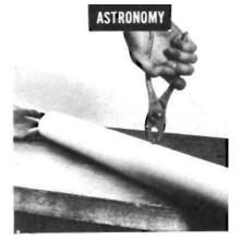
Hole is drilled at marked point in aluminum tube, right through cardboard tube. Notch a strip of wood (or bend heavy wire into loop) to hold machine-screw, which is then guided from inside tube and inserted in hole. Nut is then tightened from outside. Whole process is repeated with the second cardboard stop-tube.
