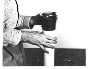
Now that objective lenses have been settled into place gingerly, the lock-ring of casing is screwed in place. No tools are used: finger-tightness only.
