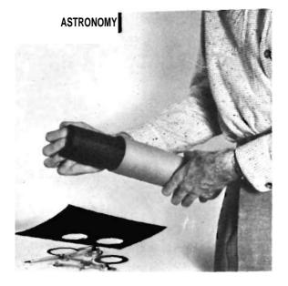
Lens-stops *are* cemented onto ends of cardboard tube, but first tube Is deadened inside with black felt paper, which also Is cemented and smoothed.
