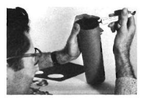
Here, stop Is being set In place. Stops are used at both ends of first tube, one or both end\* of a second (study diagram across bottom of this page).
