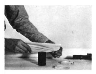
Another way to get lenses into cell is like this: using tin can or any sturdy cylinder as base, cover the cylinder with clean handkerchief, tissue.
