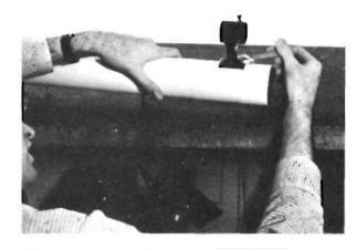
Before going on, a word of caution: NEVER DROP lenses into the casing. Follow photo instructions here. Next, fasten finder-mounting on scope-tube.
