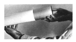
First lens-stop tube is slid into metal tube of telescope: cardboard tubes must be Just the right diameter to fit snugly, can be bought for few cents.
