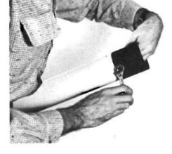
Long screws (1½ in.) should be used on previous steps, since screws will also serve to mount the telescope on tripod-head. But now attach lens-cell.
