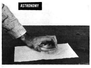
Separators provide air pocket between lenses. Place second lens carefully over one with separators. Both lenses should be resting on heavy tissue.
