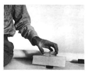
Place lens with separators in place on tissue or handkerchief. Then place other lens on top. Be sure that "flint" lens is on top. It is thickest.
