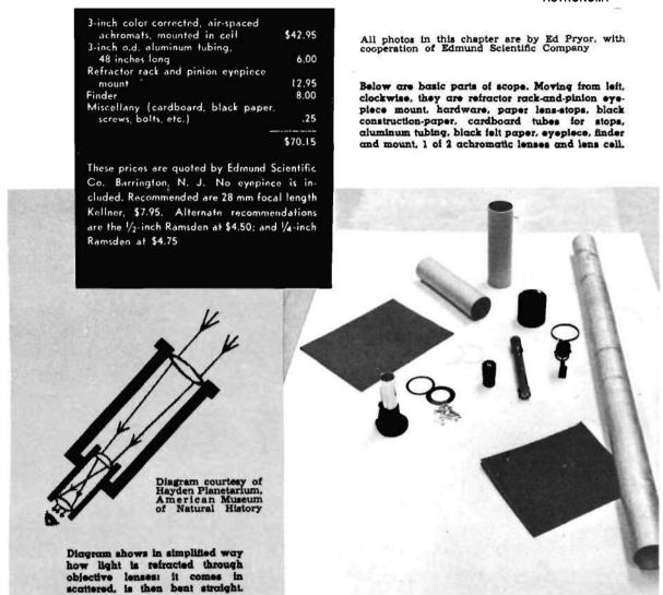
Lens-stops are of extreme importance in refractor, are cut from black paper after tracing size with compass.
