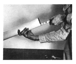
Measure distance to approximate center of inner stop-tube with long rule: hold scope-tube toward light, then peer inside and mark point on outside.
