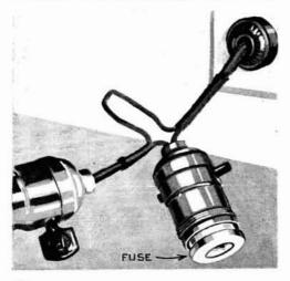
tric cord with a plug on one end and a socket on the other. Remove the insulation in the center and connect a socket containing a fuse, preferably one of low amperage, to one of the wires. To use the tester, remove all appliance wires and then plug in the tester to each one in turn. When the faulty appliance is found the fuse in the tester will blow.
