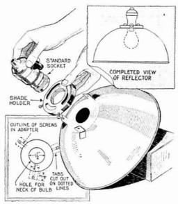
When you have occasion to attach a homemade reflector, such as the type made from an aluminum mixing bowl, to a lamp socket, try the method shown. First get a regular glass-shade holder of the type that screws onto the end of the socket. Then form tabs in the reflector and bend them up and drill them to take the screws in the holder.
