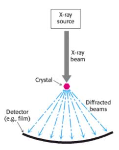
Figure 4.49. Essence of an X-Ray Crystallographic Experiment: an X-Ray Beam, a Crystal, and a Detector.
