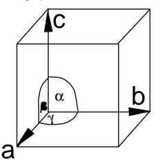
The unit cell has edges of lengths a, b, c and the angles between the edges are  $\alpha$ ,  $\beta$ ,  $\gamma$  as shown in the diagram.
